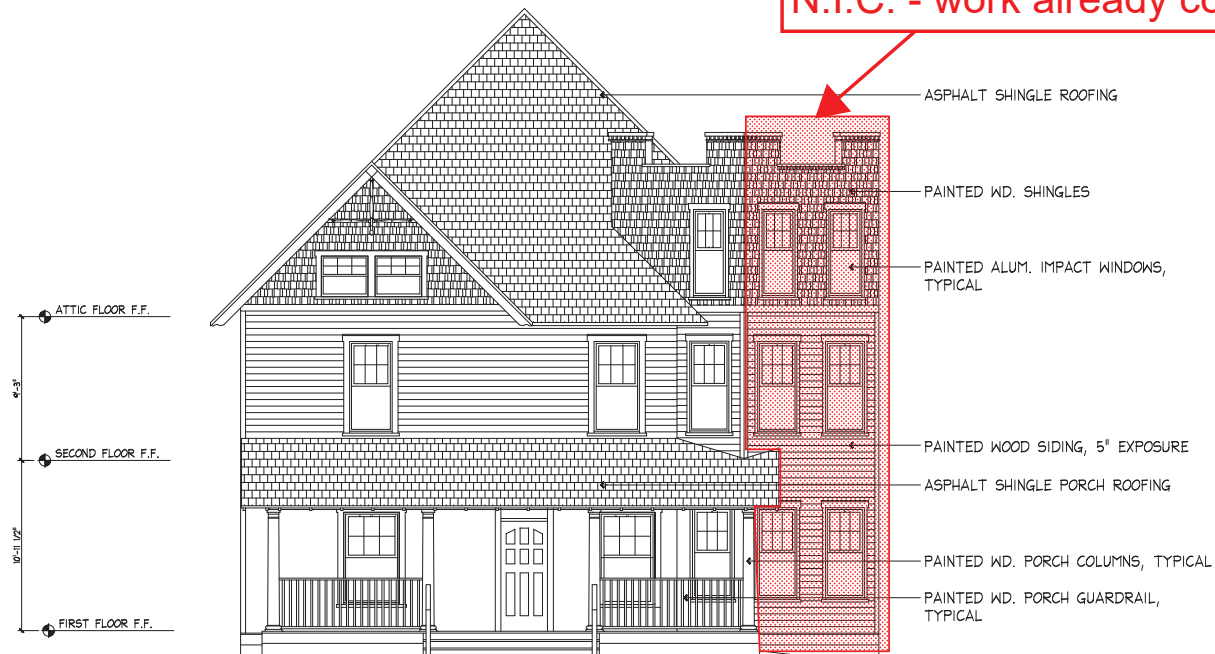
1 EX6 EXISTING NORTH EXTERIOR ELEVATION
