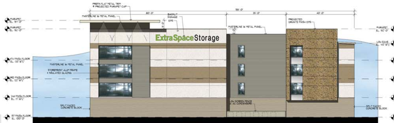
SOUTH ELEVATION SOUTH ELEVATION SIGNAGE CALCULATION 75' LP FRONTAGE 30 SQ FT + (125'-5") x 12.5 SQ FT WAIVER REQUESTED IN PBD FOR 30 SQ FT AS SHOWN SCALE: 3/32" = 1'-0"
