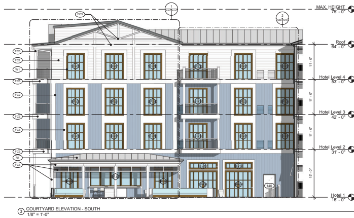
③ COURTYARD ELEVATION - SOUTH 1/8" = 1'-0"
