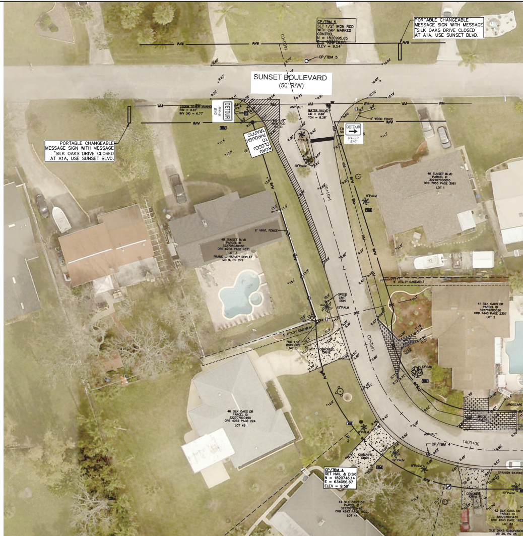
MOT PLAN FOR WET TAP AT A1A AND SILK OAKS DRIVE. (FDOT ROW)
